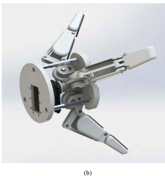
FIGURE 5. Arrangement of worm wheels connected to the actuating worm in 2D (a) and 3D (b) views.
