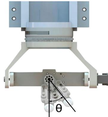
Fig. 6. Top view of the NU-Wrist robot demonstrating flexion/extension motion
