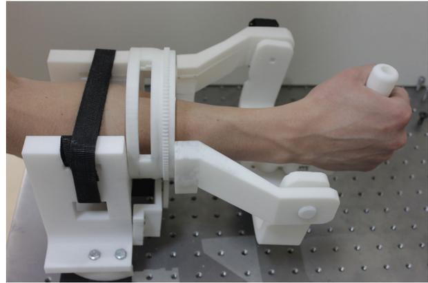
Fig. 10. A 3D printed proof-of-concept prototype of NU-Wrist rehabilitation robot tested by a healthy subject
