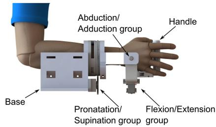
Fig. 3. Rendered side view of NU-Wrist robot with a human arm CAD model. The device can either be installed on a table or worn by user
