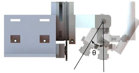
Fig. 5. Side view of the NU-Wrist robot demonstrating radial/ulnar deviation motion
