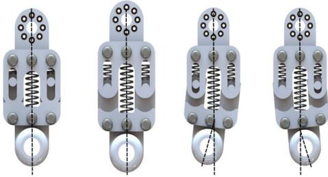
Fig. 8. Four different configurations of the compliant structure
