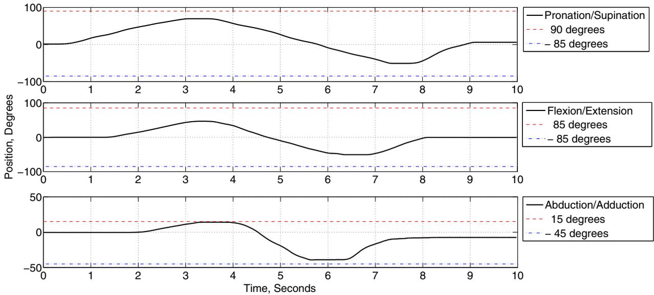
Fig. 11. Range of motions for PS, AA and FE DOFs (degrees) of NU-Wrist rehabilitation robot during active motions of a healthy subject
