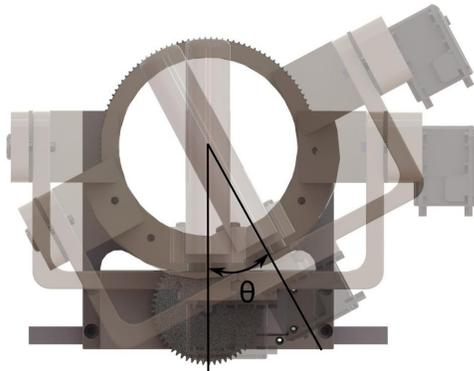
Fig. 4. Front view of NU-Wrist robot demonstrating pronation/supination motion
