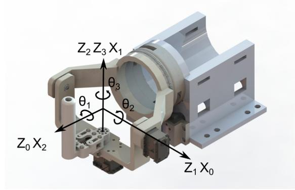
Fig. 9. Kinematic structure of NU-Wrist rehabilitation robot
